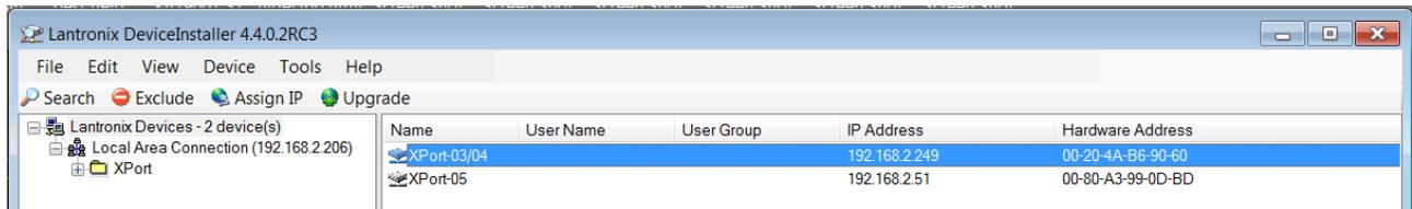
Look at the MAC address on the rear of the PSP1 and match it to one of the Xports in the list. If you only have one Xport you may assume it has the correct device and only one will be listed. Select the device in the list to highlight it. Then click on “assign IP”. The following should appear:
