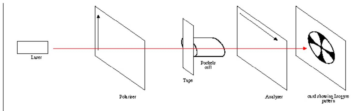
Figure 30 Modulator Between Crossed Polarisers
