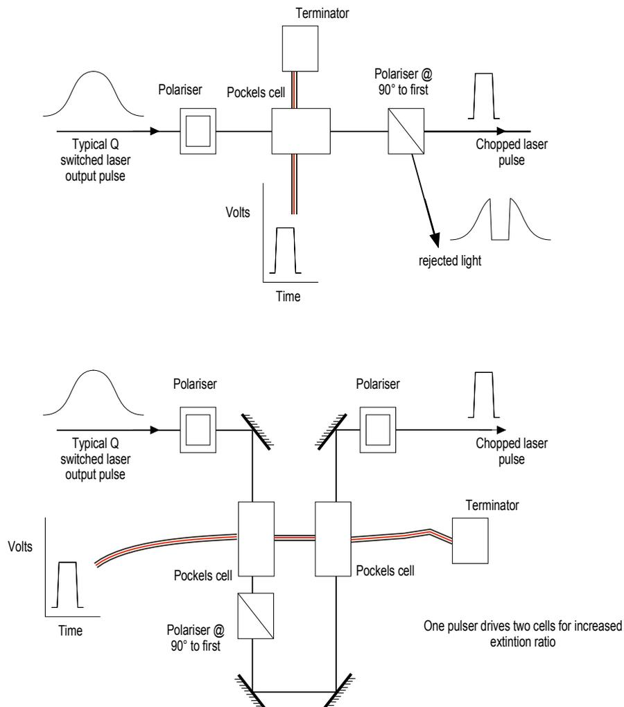
Figure 29 Some typical arrangements of the pockels cell.
