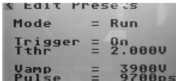
The cursor can be moved up or down using the UP and DOWN buttons. Pressing the RIGHT key on a line one allows editing of that line. For parameters that have numbers to edit the right and left keys will move among the digits. It may be necessary to edit the lower significant digits to reach the maximum or minimum permitted values. The UP and DOWN keys allow changing of the field at the cursor.
