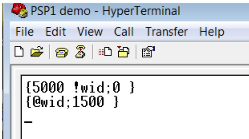
to change the width to 5000 ps first switch the PSP1 to Remote Mode on the front panel, then try again.
