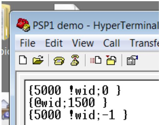
Note this time the response includes a -1, this means that the command was accepted. To check, read the width again.
