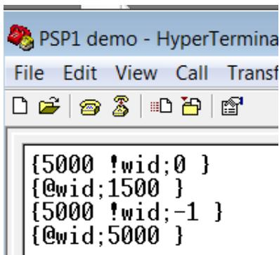
The following might be a suitable initial set up command sequence.
