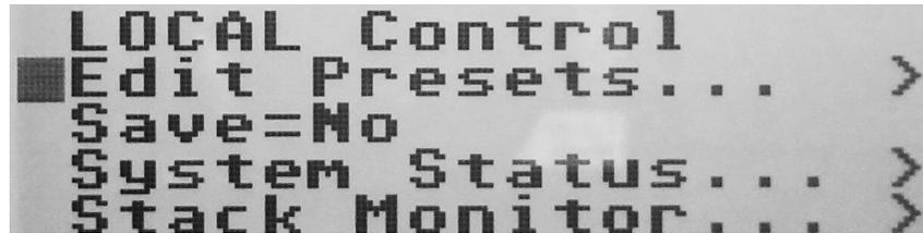
The cursor will initially be adjacent to the E of Edit. The cursor can be moved up or down onto lines 2 to 4 using the UP and DOWN buttons. Pressing the RIGHT key on line one causes the PSP1 to enter the page for the selected option.
