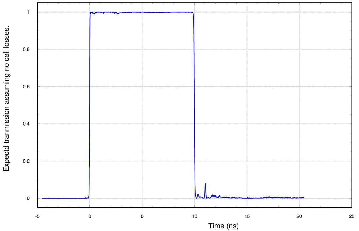
Figure 28 Expected Pockels cell response with pulser.
