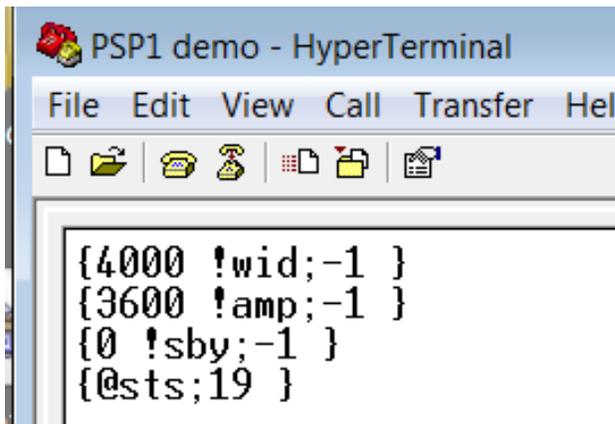
This sets the width to 4000ps, the amplitude to 3600 volts, and takes the unit out of standby. The status is then interrogated.
