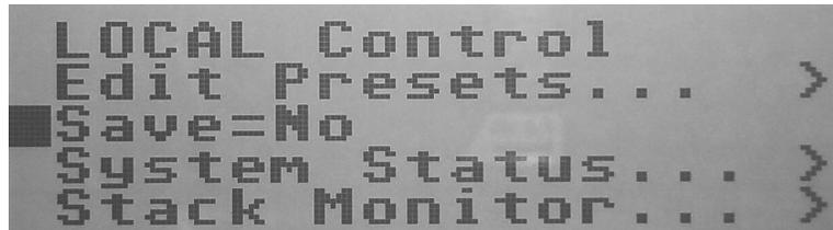
There is one editable parameter on the SAVE command. From the above position hit right to move the cursor to the “NO” then the UP/YES button to change the state and then the LEFT button to move out of the SAVE field.
