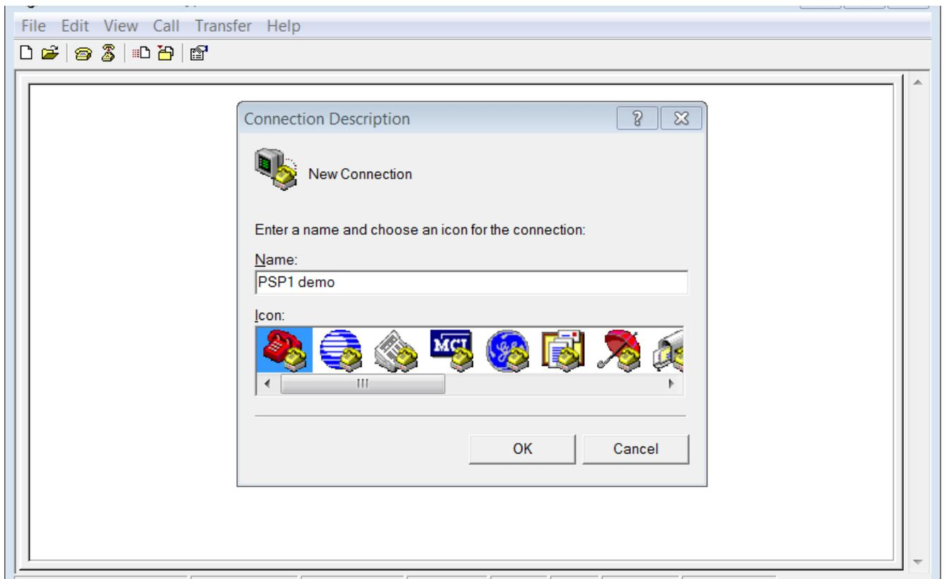
Click OK, then fill in the IP address that was set with Device Installer and set the Port Number to 10001. The connect Using should be set as shown. Click OK
