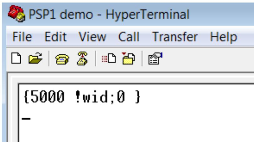
Note that this has responded with a “0” after the command. This implies that the command was not accepted. This is because the PSP1 is set to Local Mode.
