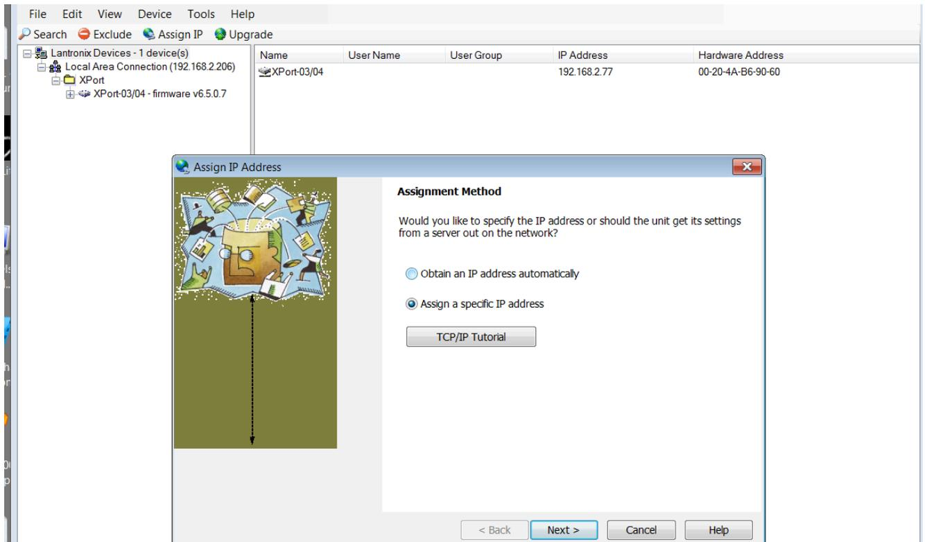
Choose whether to let the LAN router to assign an IP address or whether to set a fixed one. If you are not familiar with IP address click the link to the tutorial. If you select a fixed address you will also need to provide the subnet and gateway IP address. The following assumes that the address is obtained automatically. Select Obtain Ip address automatically and then click Next.
