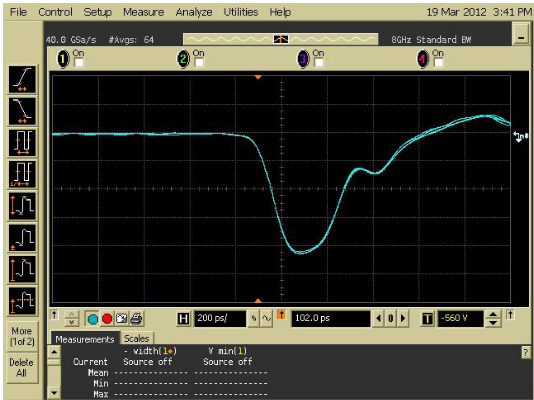
Figure 19 Main Gate output pulse waveforms 4 x 200ps modules superimposed.
