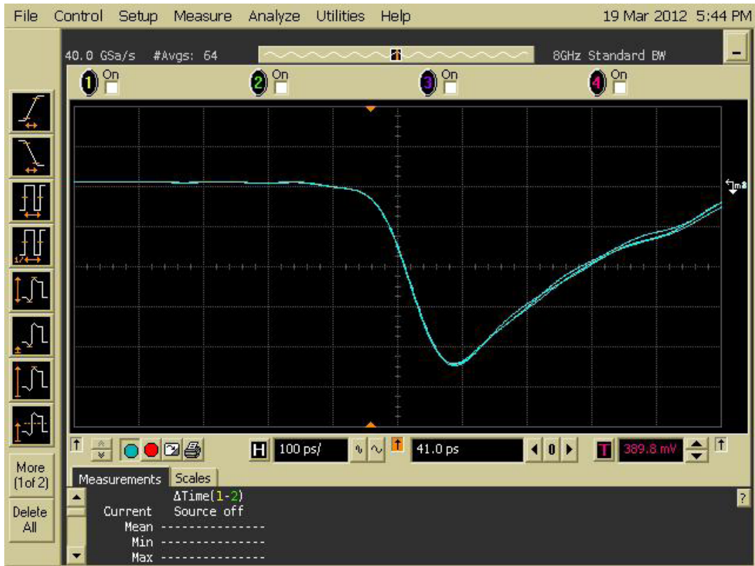
Figure 15 Main Gate output pulse waveforms 4 x 100ps modules superimposed. High voltage setting. Peak is at is -4530 volts.
