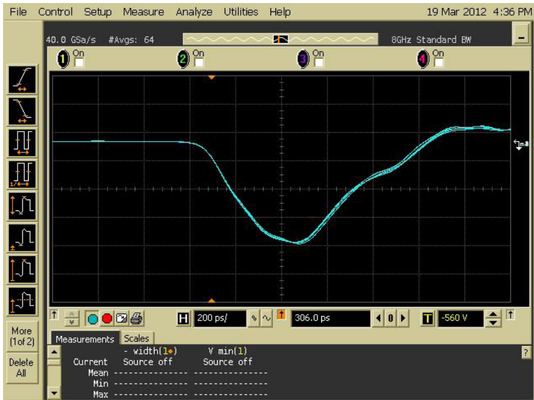
Figure 21 Main Gate output pulse waveforms 4 x 400ps modules superimposed
