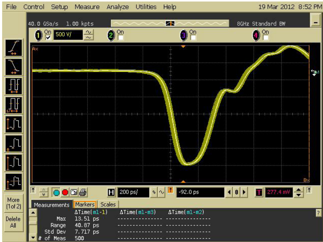
Figure 26 The overall system jitter when driven optically Range 40.87ps, SD 7.717ps
