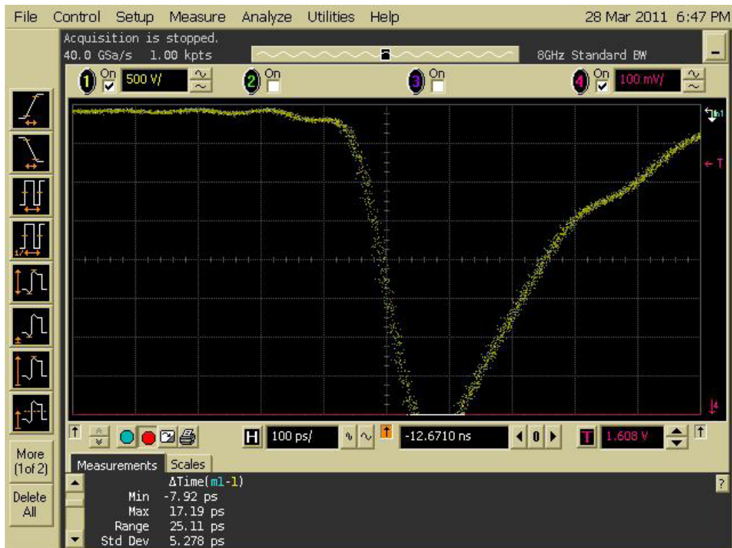
Figure 27 The overall system jitter when driven electrically Range 25.11ps SD 5.278ps
