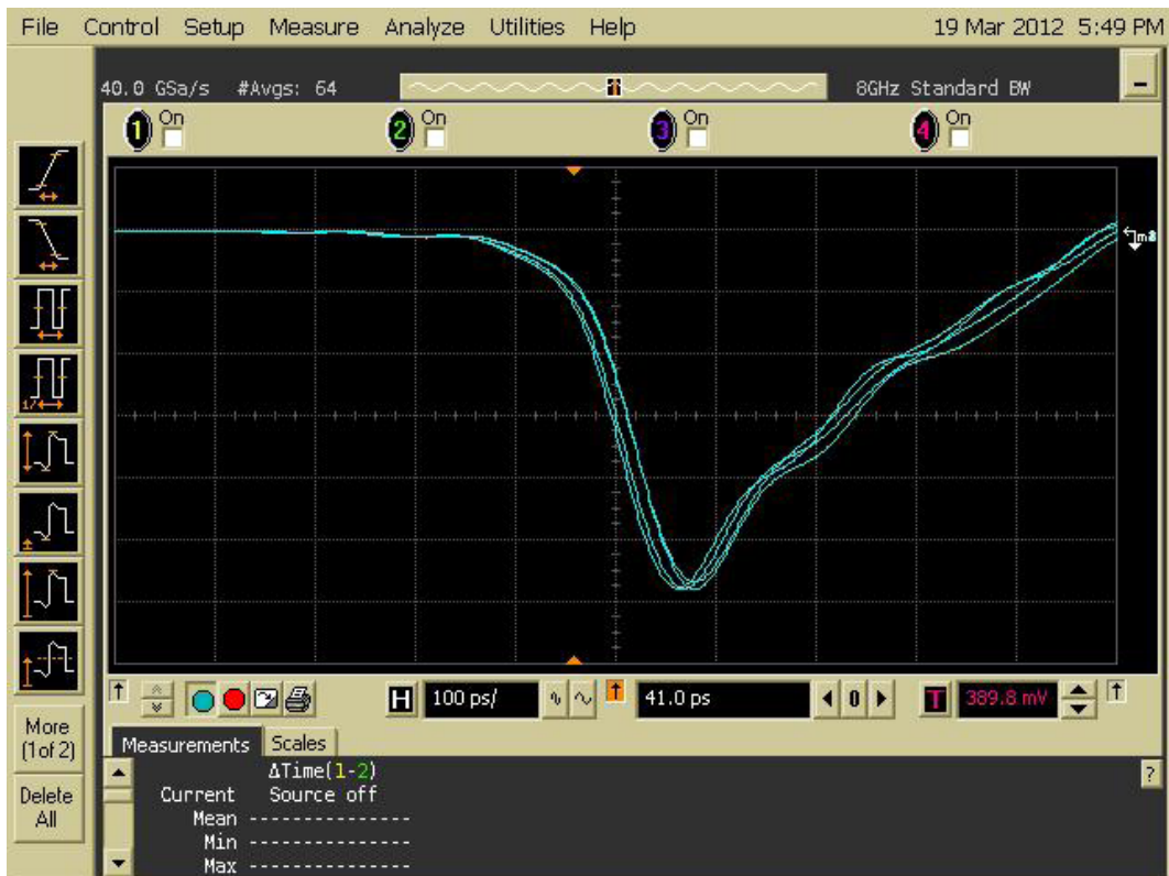
Figure 16 Main gate output pulse wave forms 4 x 100ps modules showing relative timing. Low voltage output. PRM timing differences are shown for synchronised raw pulses. Peak voltage ~ 2.8kV
