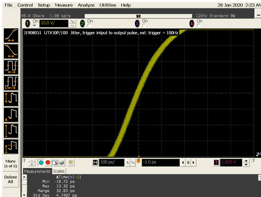
Figure 11: Pulse jitter, Trigger input to Pulse output, Ext. trigger
