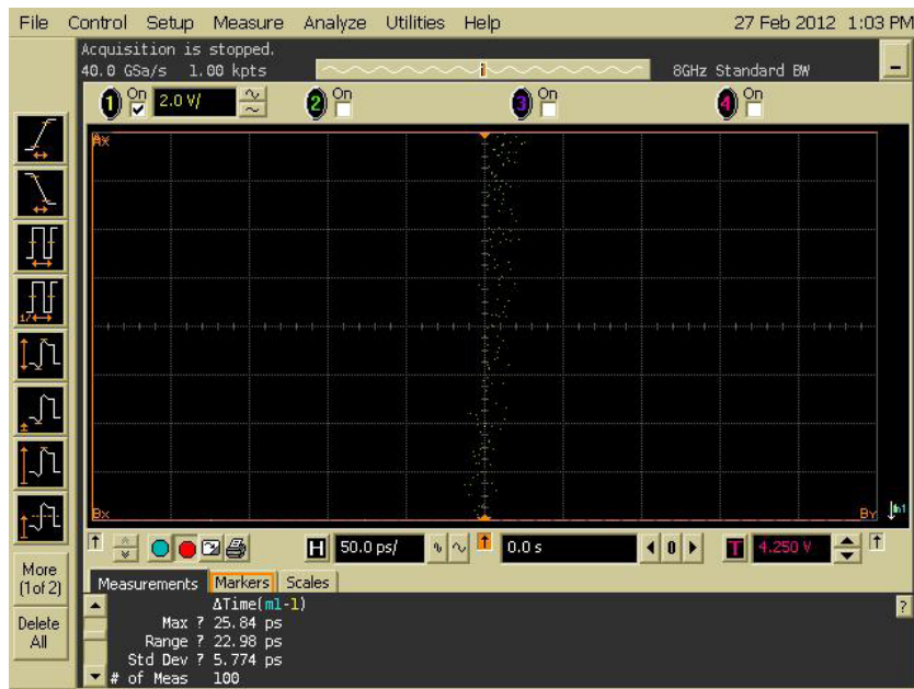
Figure 39 Sweep 0 jitter Range 22.98ps; standard deviation 5.774ps
