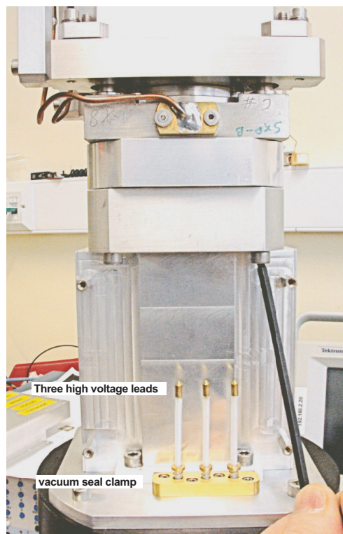
Figure 8 Tighten the four M5 screws to clamp the MAX module
