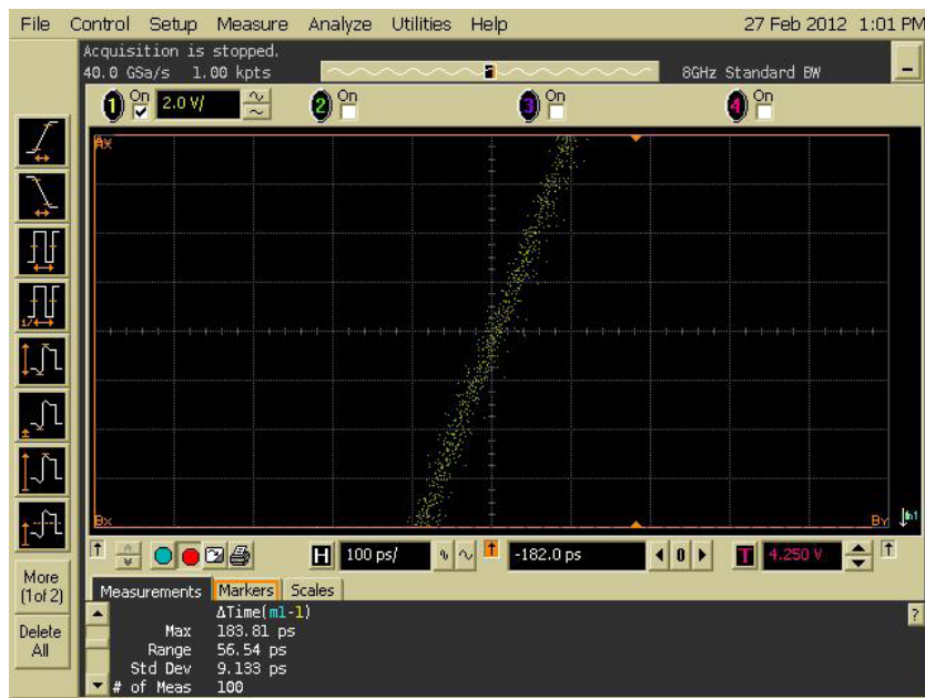
Figure 40 Sweep 5 jitter Range 56.54ps; standard deviation 9.133ps
