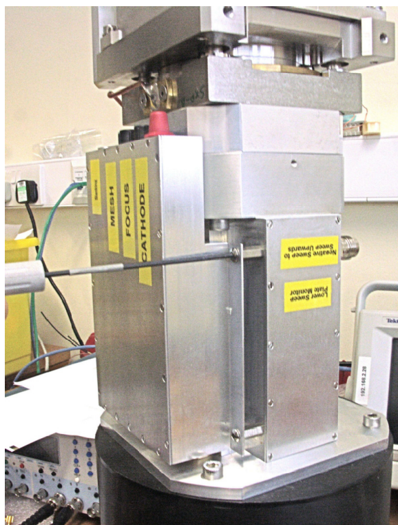
Figure 7 Remove the four M3 screws to loosen the Clamp box. Then lift the clamp box off the three high voltage leads very carefully and without tugging.
