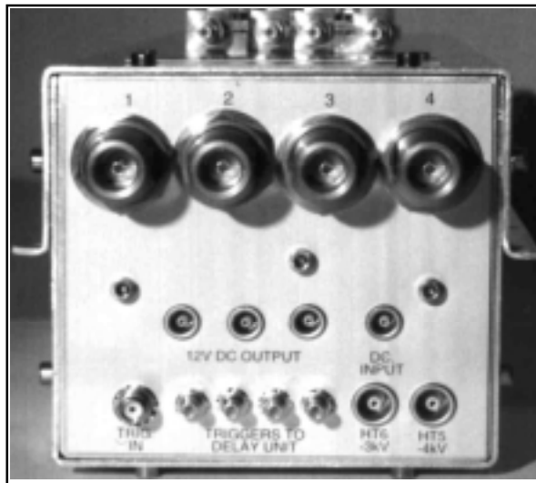
The pulser bulkhead showing trigger input, HTs, and trigger loop throughs, DC inputs and outputs, to access the on board regulator, and the main pulse outputs.
