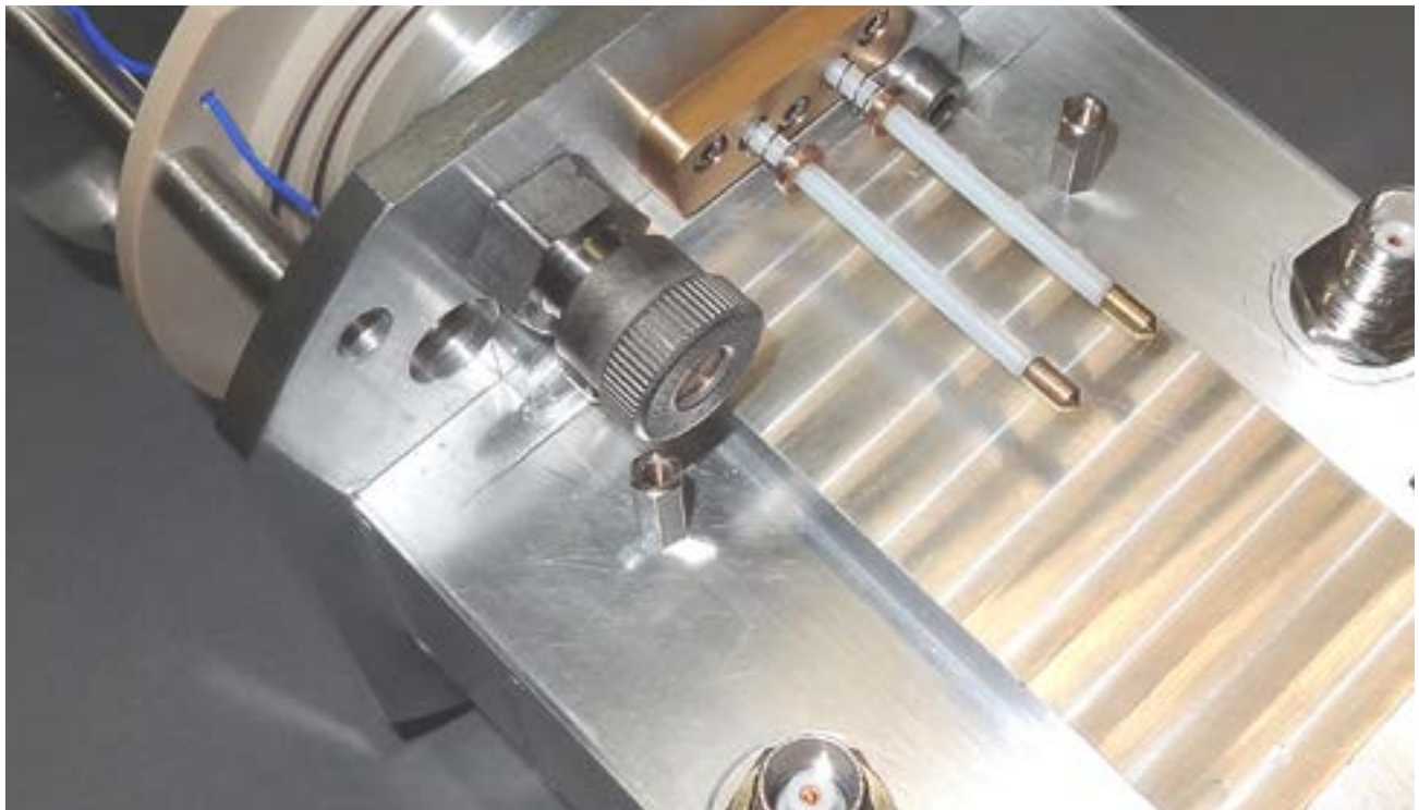
Figure 8 With the connector boxes removed Take care not to damage the four high voltage leads or to lose the washers and springs. Check that the brass end connections are in good order and well soldered to the cables. Note that these cables have copper inner conductors and are not as robust as most semirigid cables.
