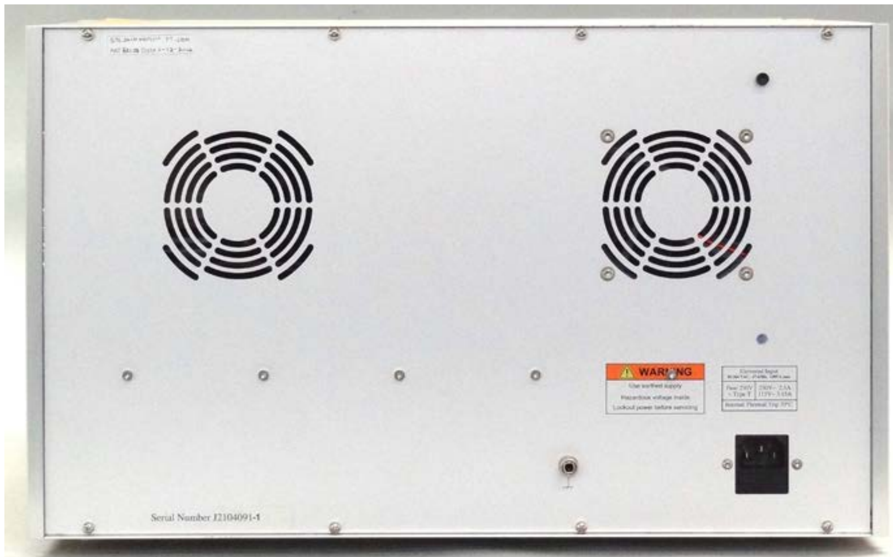
Figure 11 Rear panel of the rack unit The EEPROM write protect button is at top right
