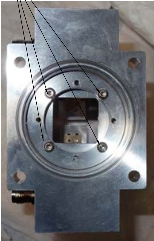
Figure 5 Scraper ring mounting. View into rear end of streak tube before fitting the sensor. The scraper ring can be loosened and moved. If necessary it can be mounted in the reverse direction using the second set of threaded holes. There is no forced alignment of the orientation. this should be set by “eye” or measured.
