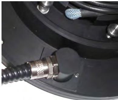
Figure 12 The Intensifier cable gland can be rotated
