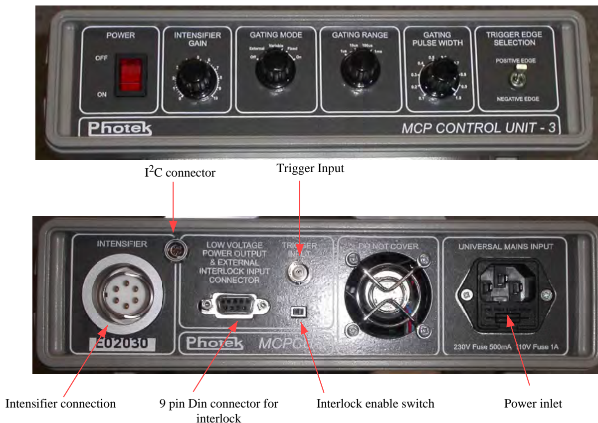
Figure 11 The Intensifier power supply panels
