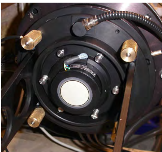
Figure 9 Intensifier mount flange with knurled nuts and the lens assembly removed
