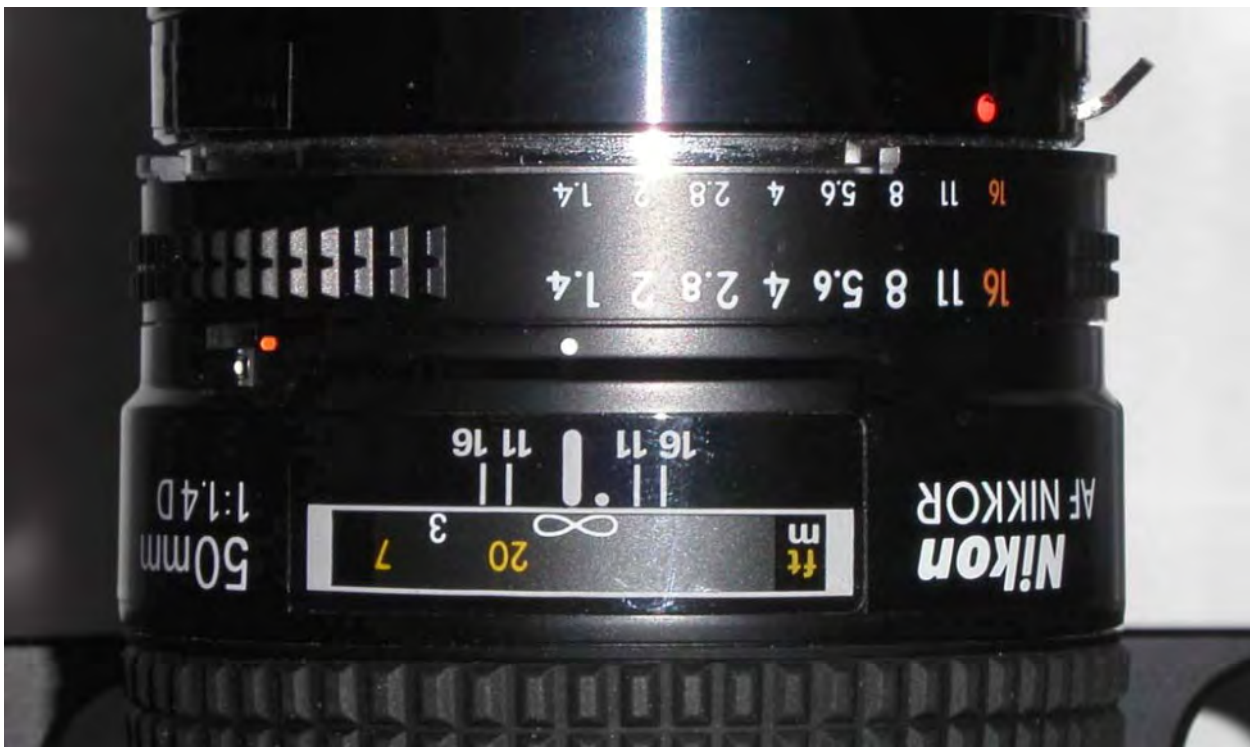
Figure 23 The second lens showing the focusing ring and the aperture control Note there is also an aperture control on the first lens. The focusing ring on the first lens has no effect on the focus.
