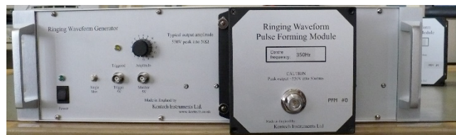
Figure 6: PFM secured in place
