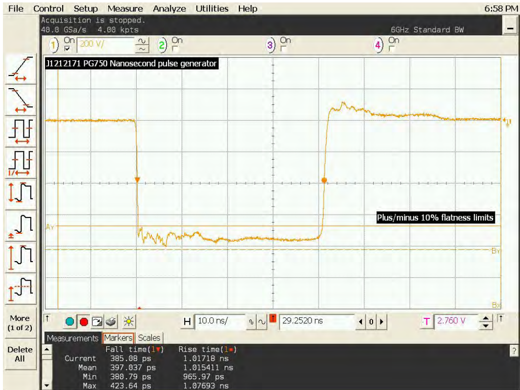
Figure 7 Output at maximum amplitude and pulse width showing flatness.
