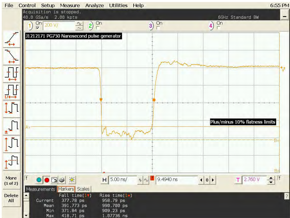
Figure 8 10ns pulse parameters showing rise and fall times at max amplitude.
