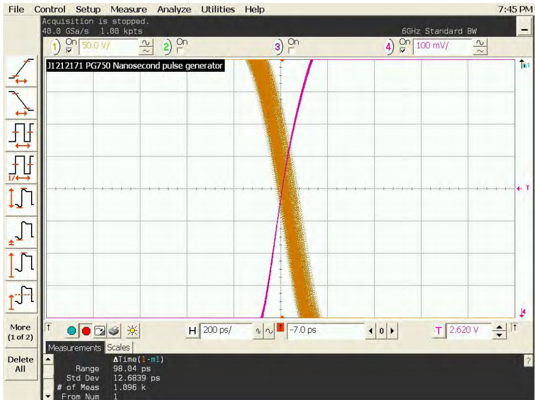
Figure 6 Output timing uncertainty, jitter at 200ps/div. RMS jitter ~ 15.4ps.
