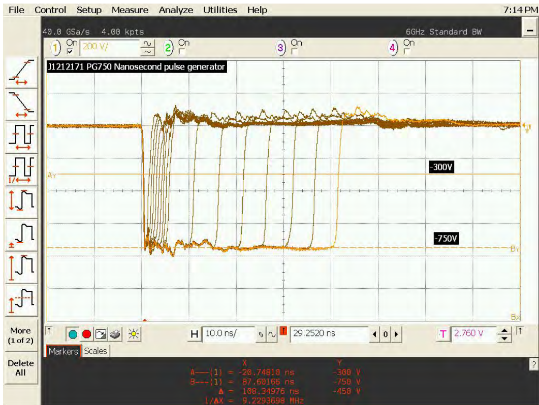
Figure 3 Variation of output pulse length
