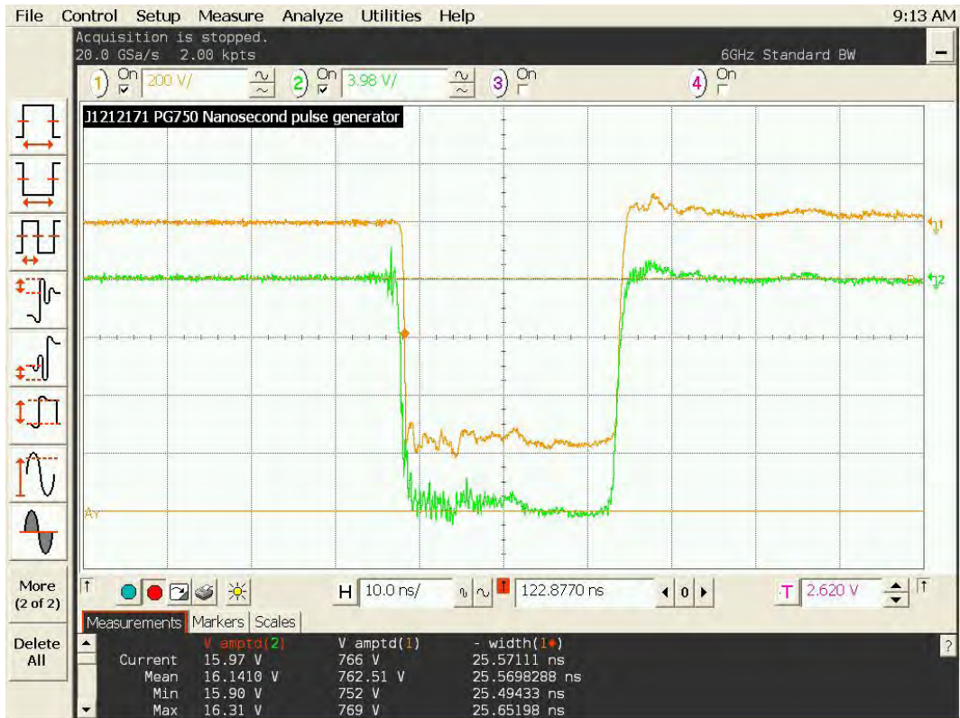
Figure 5 Comparison of monitor output (green) to main output
