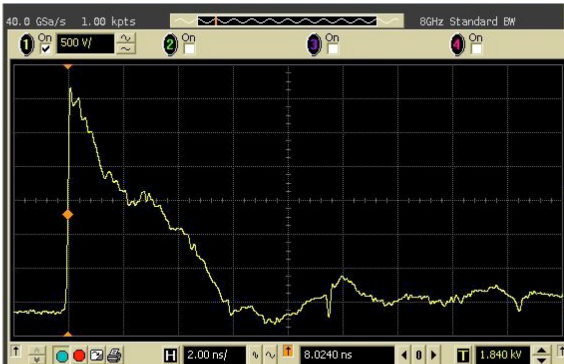
Figure 6 The long time history of the pulse at maximum amplitude. This is with the extension lead between the pulser and the Suicide “T”. The small negative spike at ~9.5 ns into the pulse is due to the lack of complete cancellation of the pulses in the two side arms of the Suicide “T”.
