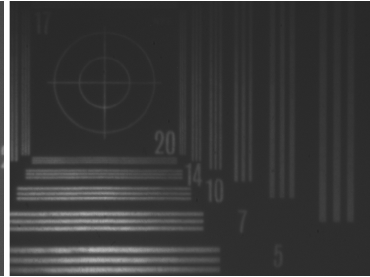
Standard two magnets Red light Gating 200ps 20LP/mm is 33.9 LP/mm on cathode.
