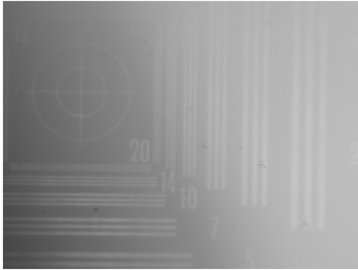
Extra magnet Red light Gating 200ps 20LP/mm is 33.9LP/mm on cathode.
