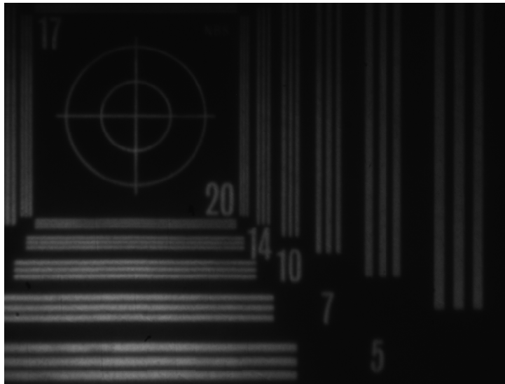
Standard two magnets Red light DC 20LP/mm is 33.9 LP/mm on cathode.
