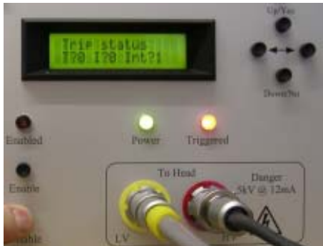
Figure 13 If the system trips, push the Disable button to interrogate the software for the cause.
