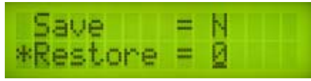
Figure 7 Save and restore settings. On power up settings in set 0 are used.
