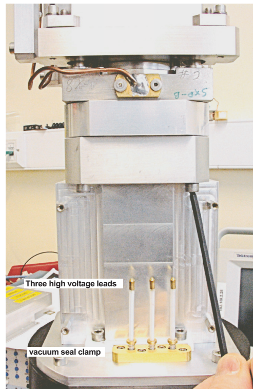
Figure 11 Tighten the four M5 screws to clamp the MAX module
