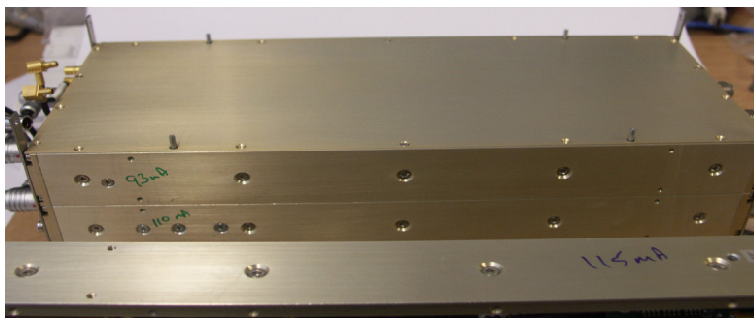
Figure 4 Split modules showing the mounting pins.
