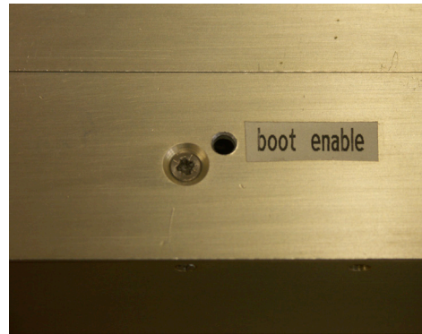
Figure 16 The boot enable access hole is located on the top of the control unit
