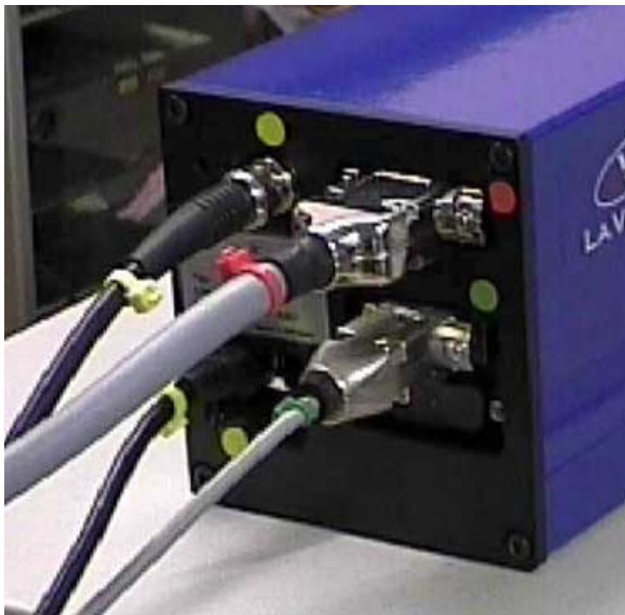
Figure 10 The rear of the CCD head, showing the leads fitted.
