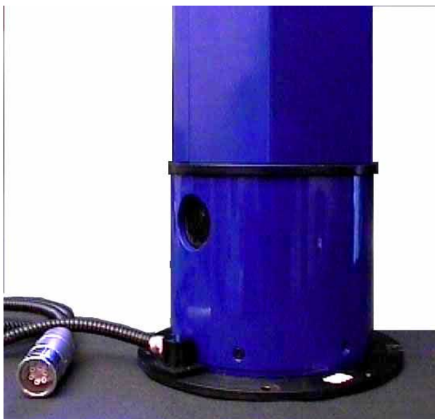
Figure 11 The CCD head, showing the air flow ports
