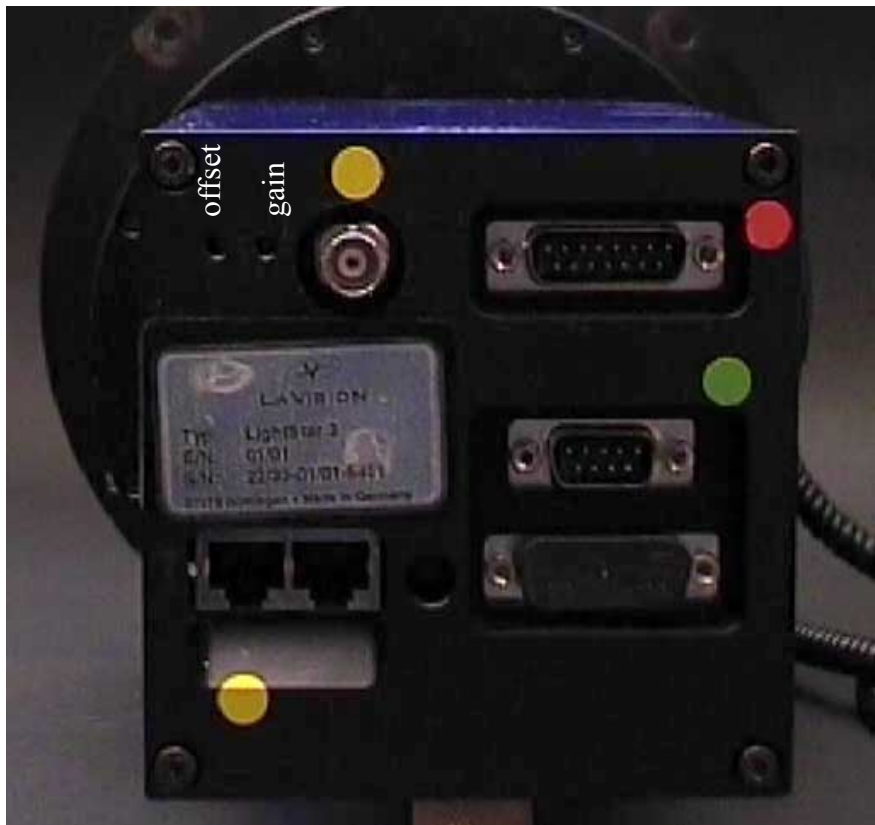
Figure 9 The rear of the CCD head, showing the gain and offset controls
