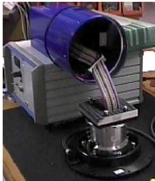
Figure 19 The insides of the CCD head
