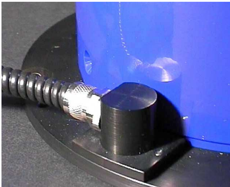
Figure 59 The Intensifier cable gland. It may be rotated by slackening the screws underneath.
