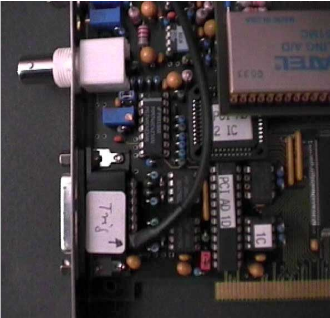
Figure 58 The internal trigger lead to the A to D convertor
