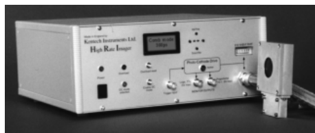
The Kentech HRI (High Rate Imager) Optical image modulation to 1GHz, gate widths to 300ps at 110MHz repetition rate
