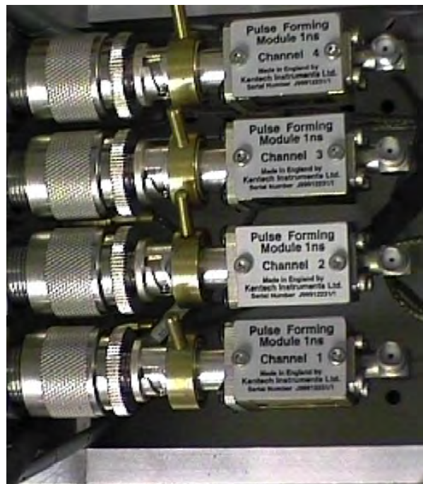
Figure 7 1ns modules fitted
