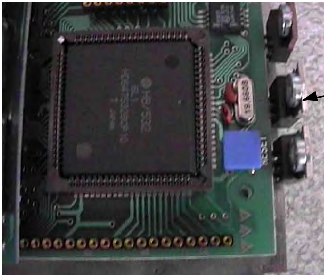
Figure 23f Make sure the regulators are not bent down before re-assembly
