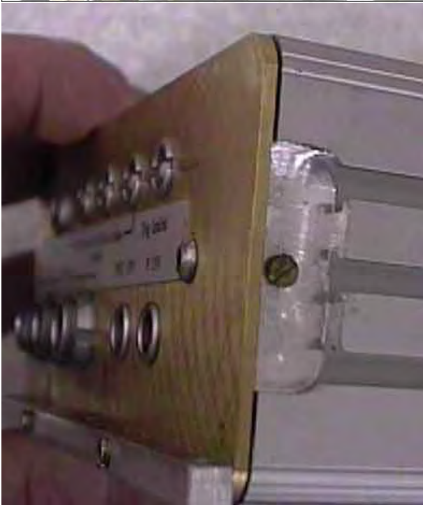
Figure 23c Remove the three screws holding the connector panel.
