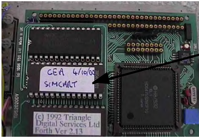
Figure 23e Locate the EPROM and replace. Note the orientation of the chip
