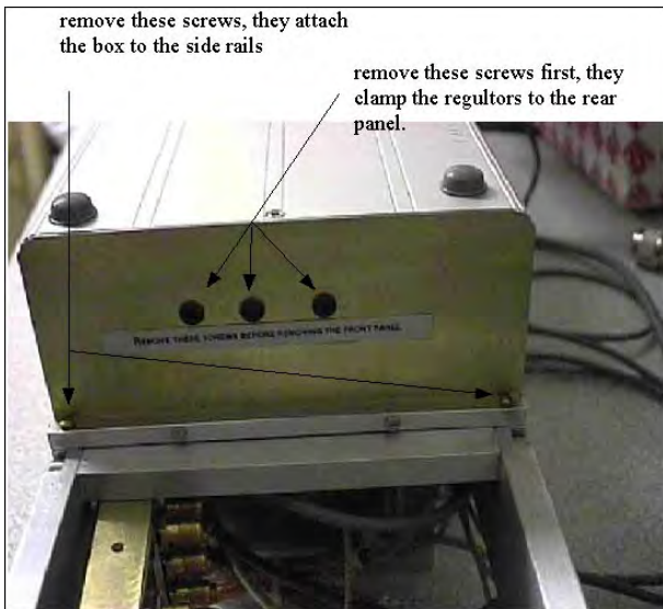
Figure 23b Remove the regulator clamp screws and the box fixing screws
