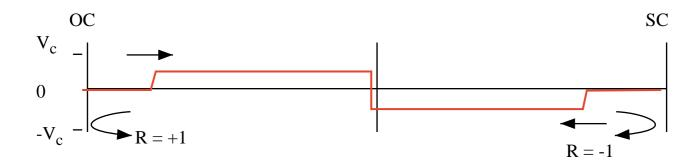
When the edges return to the load we have to consider the contribution to the load voltage from each and the splitting of the two edges into four.
